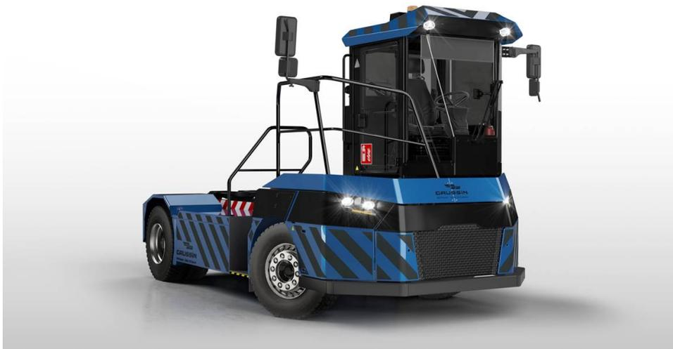
The GAUSSIN APM H2 75T, soon to be tested (spring 2022) at the Montoir container terminal
