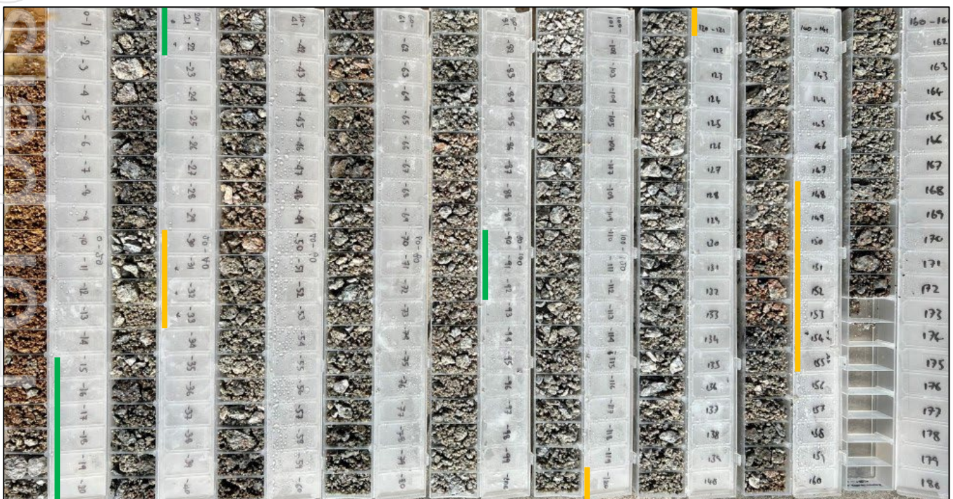
Figure 8. 22BKRC005 chip trays displaying high (red), moderate (yellow) and minor (green) sulphide abundance.
