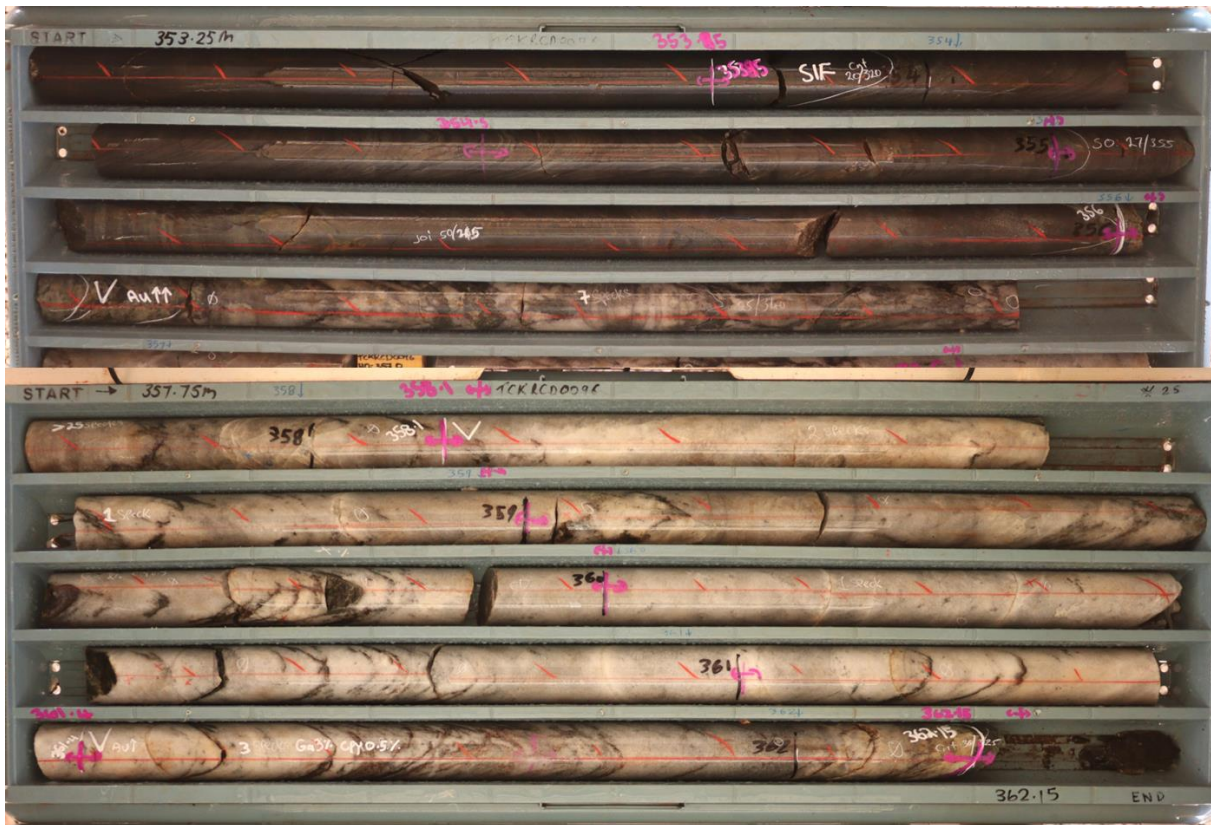
Figure 3 - TCKRCD0096 353.25m to 362.15m core photos showing vein style mineralisation
