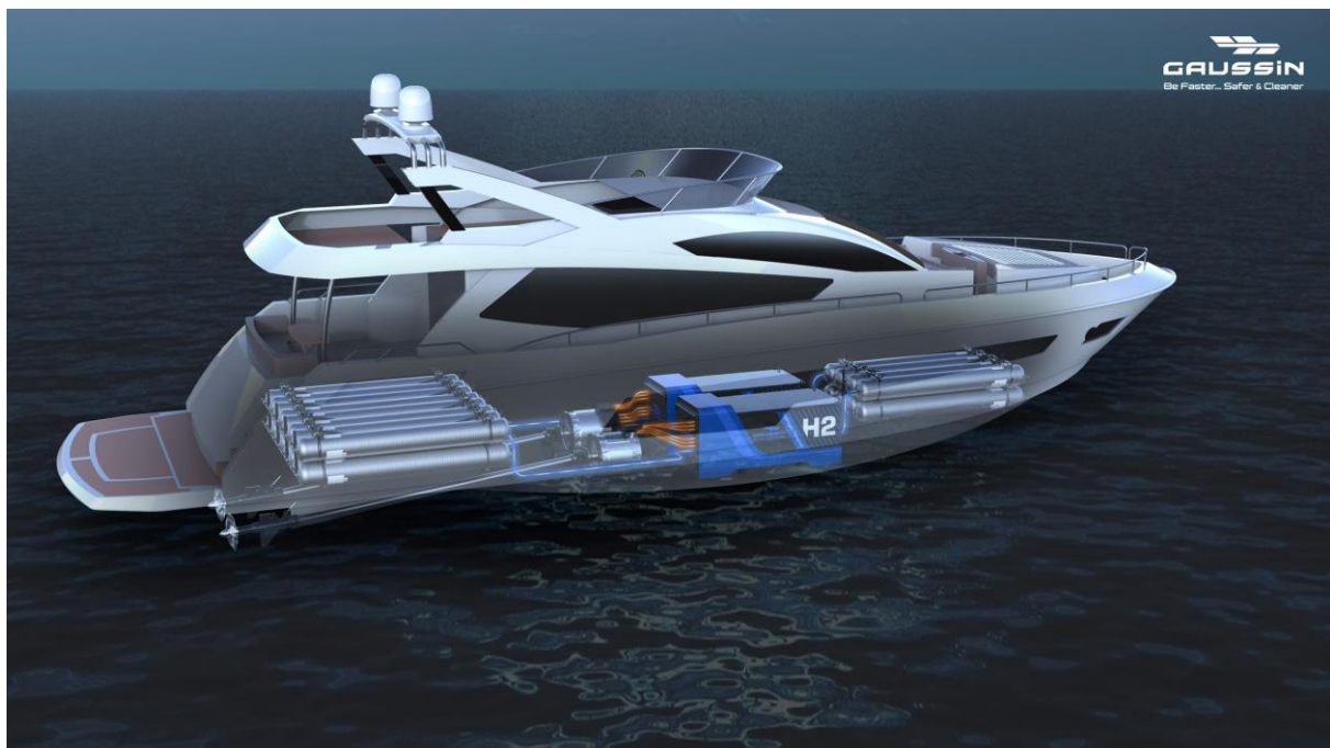
Full hydrogen system for a zero-emission boat
