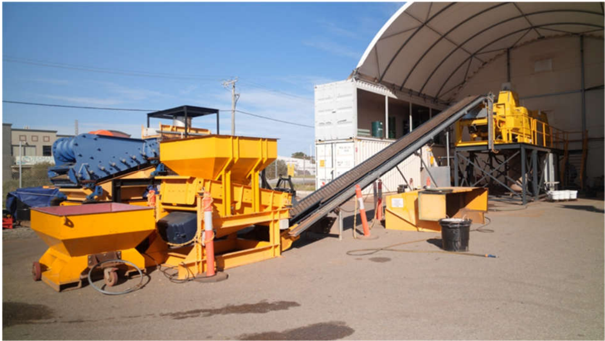
Figure 2: Ore sorting facility used during testwork is the same size proposed for use at Kayelekera
