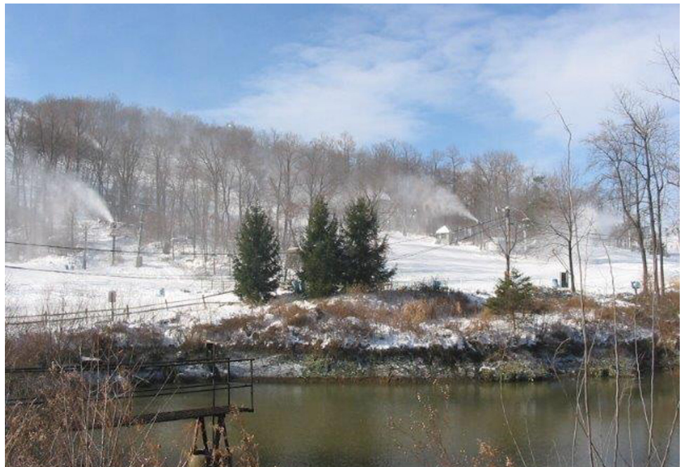
This storage pond used for snowmaking is an eligible structure and the project’s consumptive use mitigation fee will be reduced when the amount of pond evaporation is removed from its use calculation.
