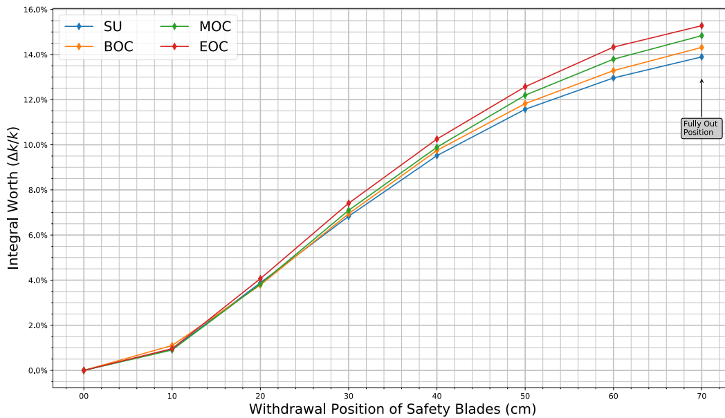
Figure 25. Integral reactivity of the safety blades in the cycle states.
