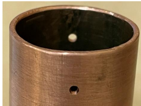
Figure 8. Pressure taps bored by end milling on a test piece.
