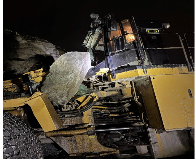
A large rock from the collapsed highwall crushing the FEL front cab pinning the miner's legs under the dash.
