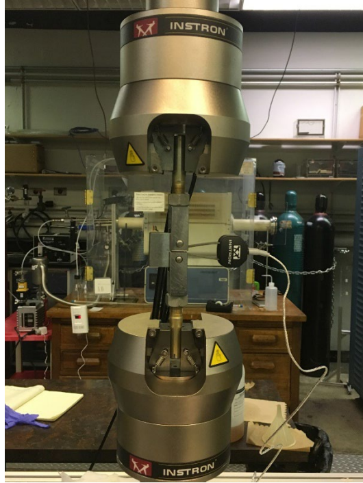
Figure 49. Compact tension fracture toughness test showing COD clip gauge
