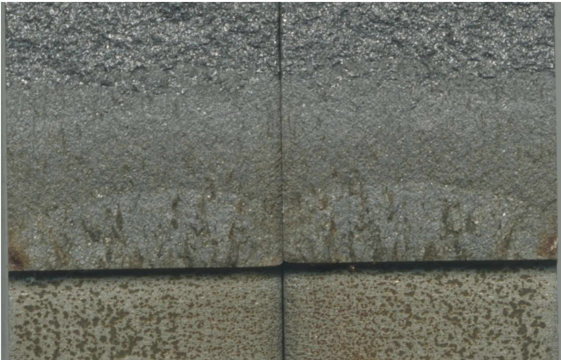
Figure 70. Fatigue/fracture surface for HH 3A tested at R=0.33
