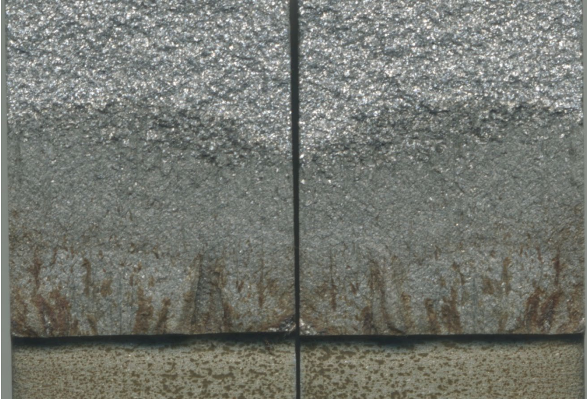
Figure 69. Fatigue/fracture surface for HH 3B tested at R=0.1
