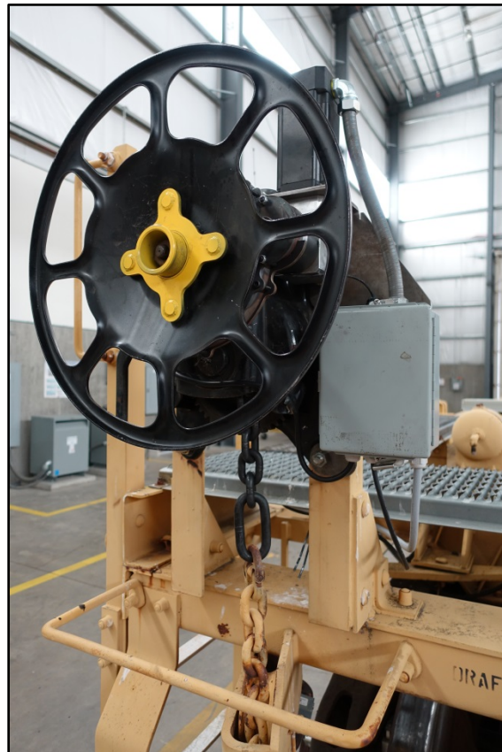
Figure 8. EDHB on well car during in-lab wireless short train testing
