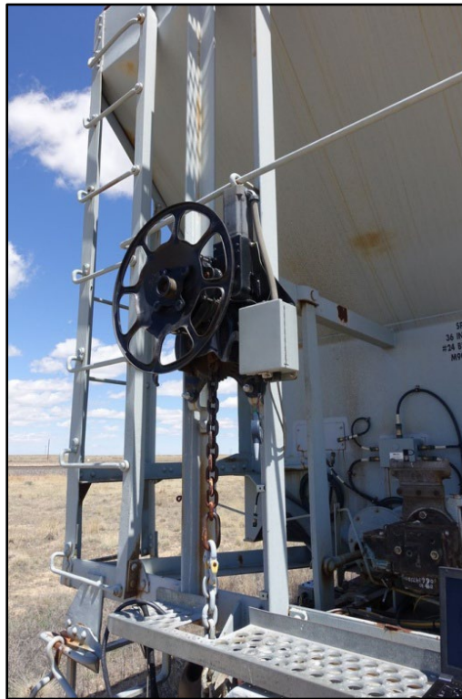
Figure 1. An SA designed and developed EDHB under test at Transportation Technology Center, Inc. (TTCI)
