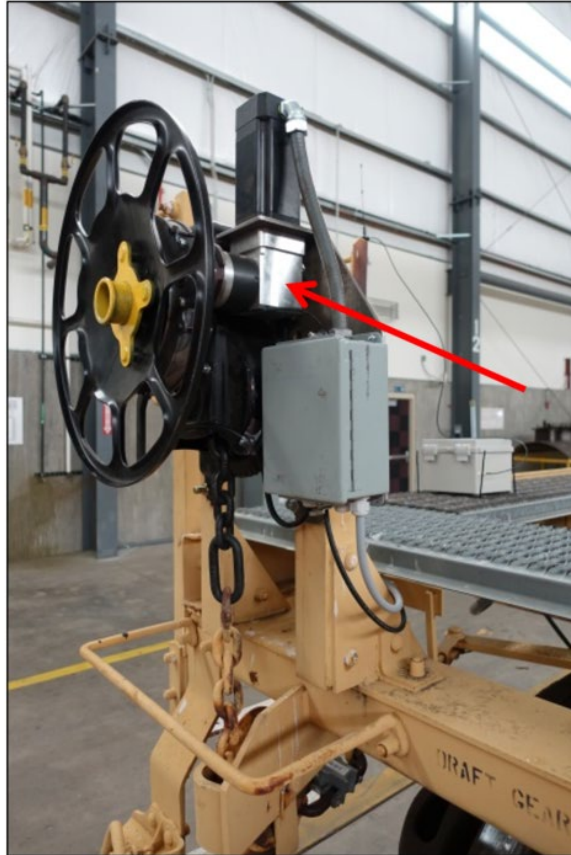
Figure 5. New gearbox installed in system
