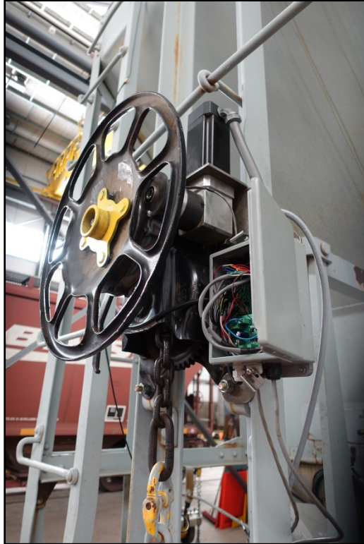
Figure 7. EDHB installation on the covered hopper prior to short train test
