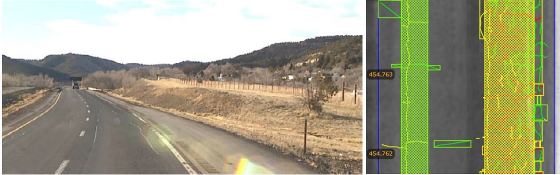
A. 2020 Fugro images: forward image on the left and downward image on the right.
