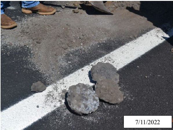
Figure 77. Photo. Unbound granular layer extracted from the northbound lane; I-25, Colfax County, New Mexico.
