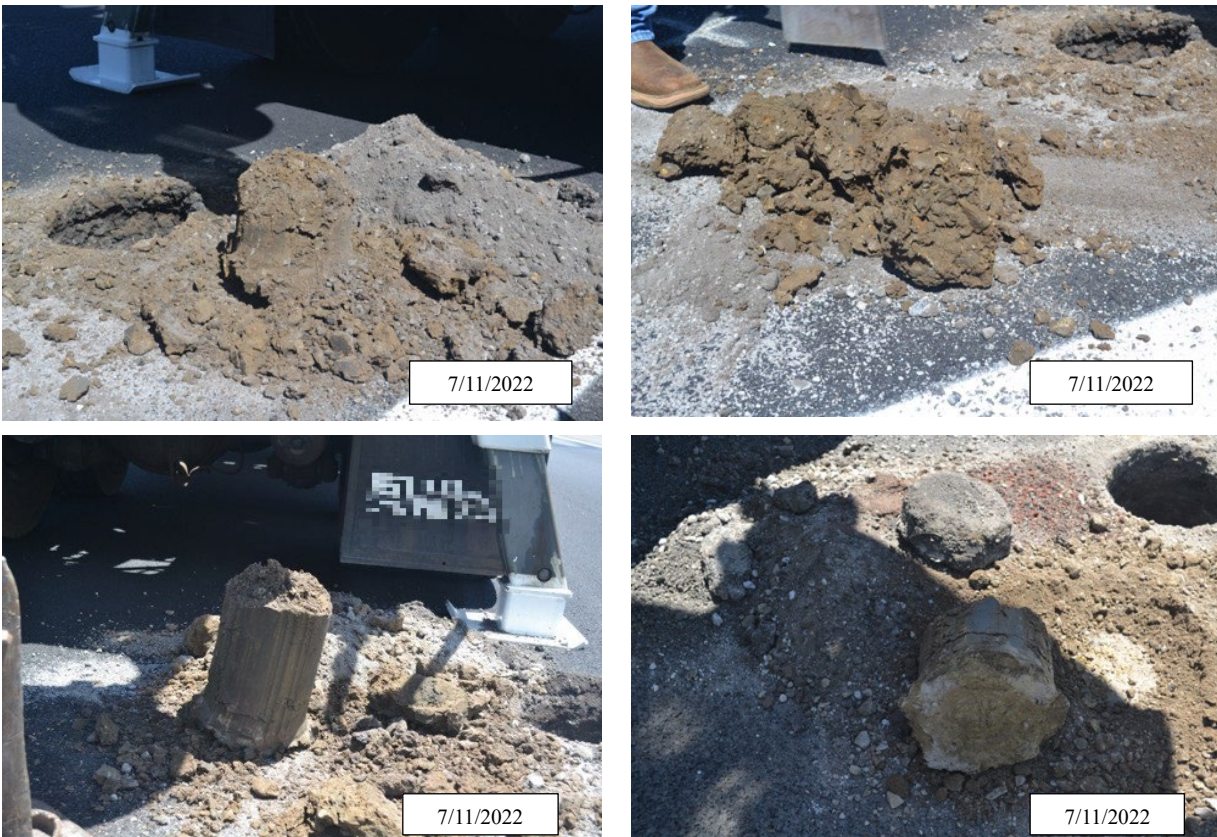
Figure 76. Photo. Subgrade samples collected from both directions; I-25, Colfax County, New Mexico.
