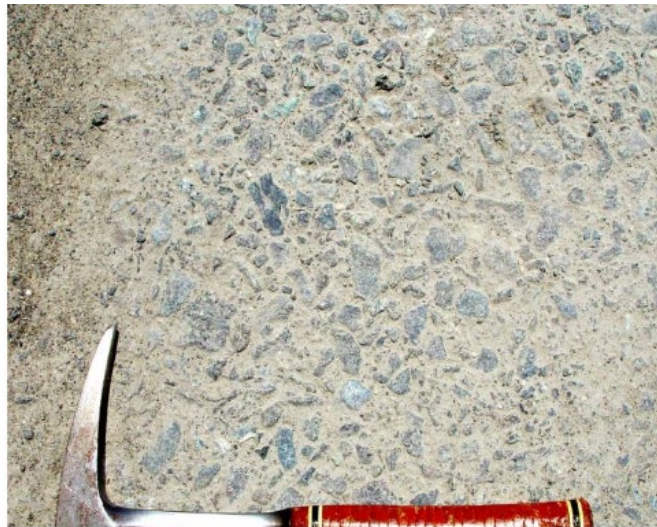
A. Slush compacted G1 layer at an HVS site.
