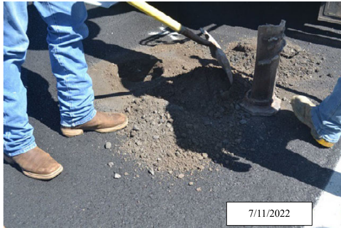
Figure 77. Photo. Unbound granular layer extracted from the northbound lane; I-25, Colfax County, New Mexico.
