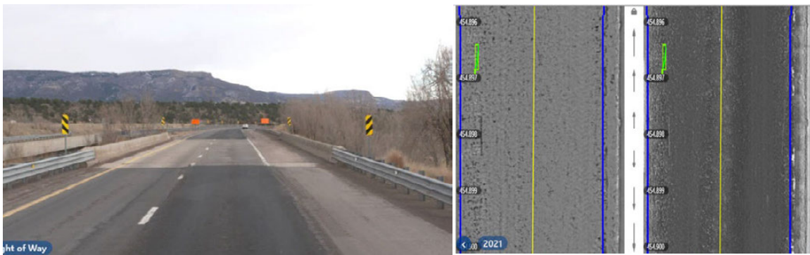
B. 2021 Fugro images: forward image on the left and downward image on the right.
