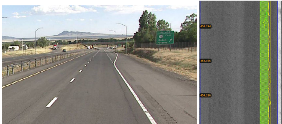
A. 2020 Fugro images: forward image on the left and downward image on the right.
