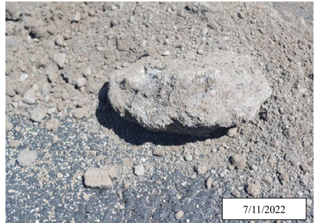
Figure 77. Photo. Unbound granular layer extracted from the northbound lane; I-25, Colfax County, New Mexico.
