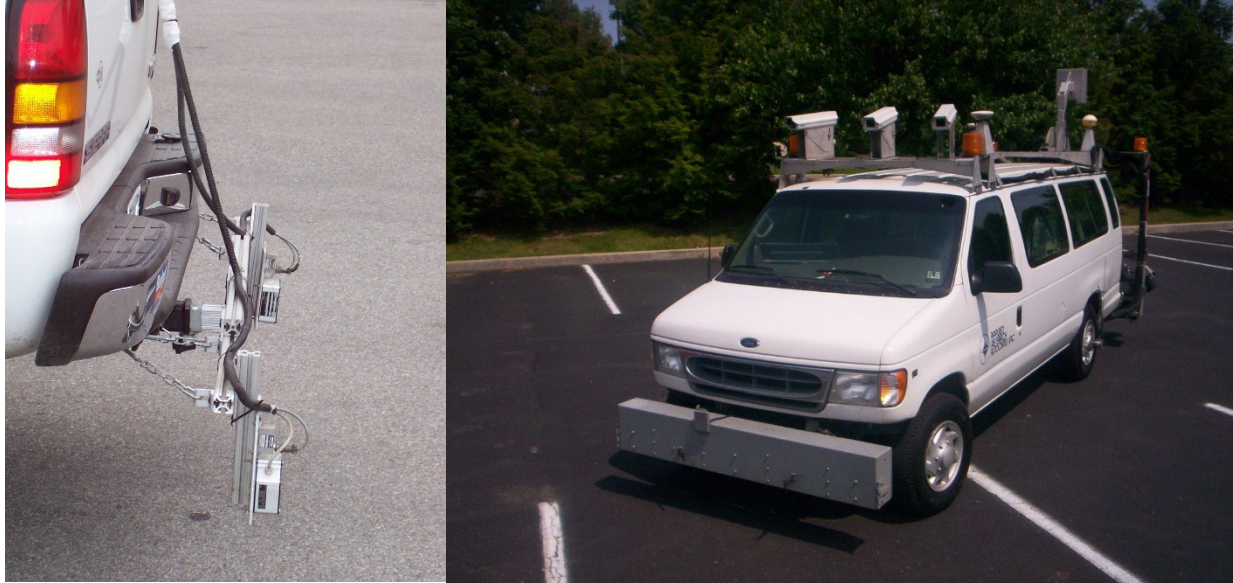
Figure 3. Photo. 2D Automated Fault Measurement (AFM) equipment based on High-Speed Inertial Profiler (HSIP).
