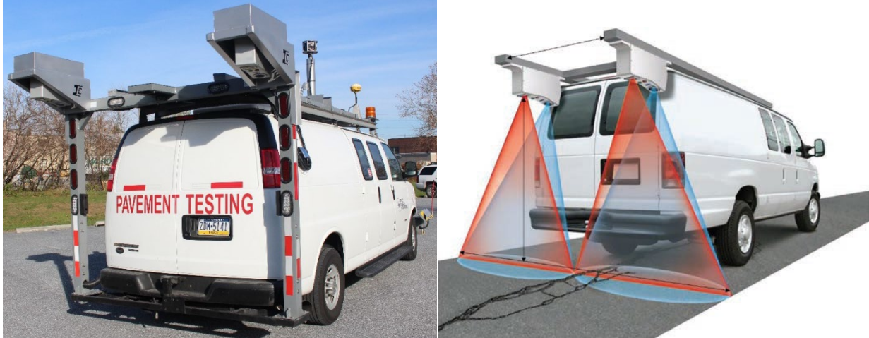
Figure 7. Photo and Illustration. 3D Automated Fault Measurement (AFM) equipment.
