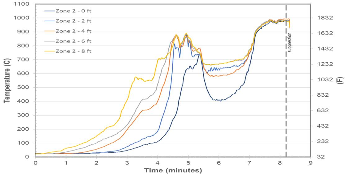
**Figure 14. Temperature in Zone 2 at Different Elevations**
