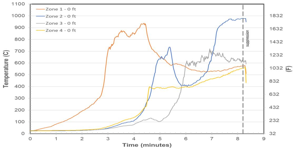
**Figure 13. Temperature at Floor Level for Zones 1-4**
