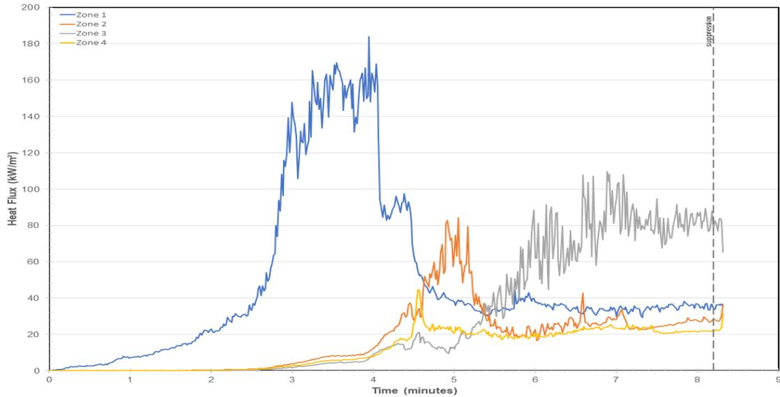
**Figure 15. Heat Flux at the Floor Level for Zones 1-4**
