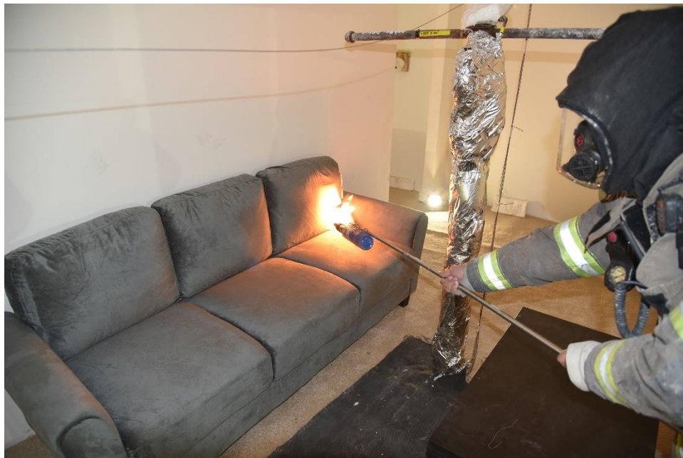
Figure 18. Ignition package ignited using open flame from butane torch (360086_1305186.jpg)
