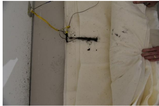
Figure 11. Cartridge heater location for Test 1 (360082_1304928.jpg)
