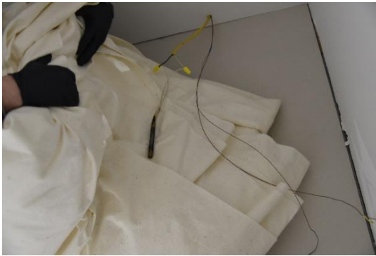
Figure 10. Cartridge heater location for Test 1 (360079_1304744.jpg)
