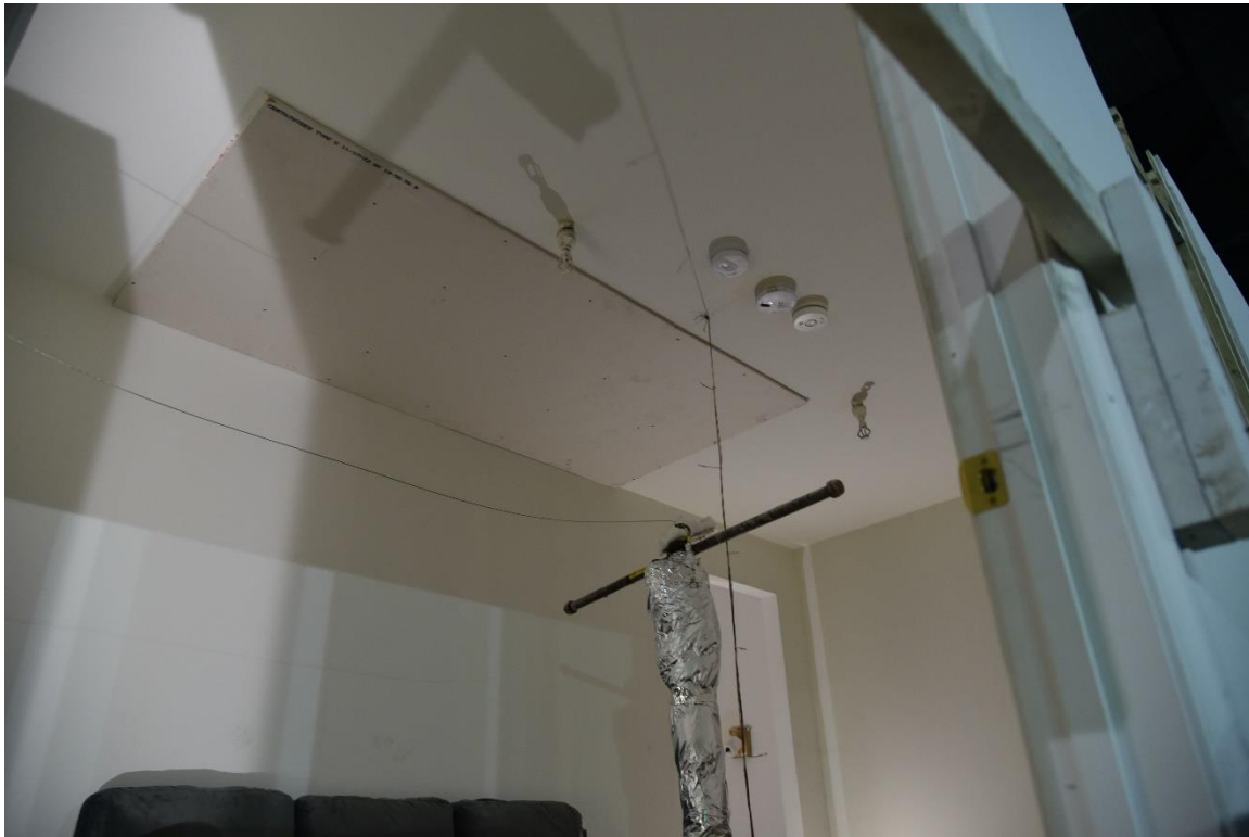
Figure 3. Extra section of gypsum wall board attached to ceiling above the sofa for the flaming fire tests (360086_1305181.jpg)
