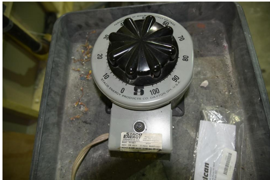
Figure 9. Variable transformer (360079_1304639.jpg)
