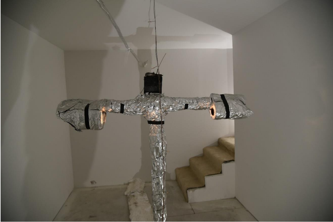
Figure 21. Instrumentation stand for tenability measurements (360086_1305132.jpg)
