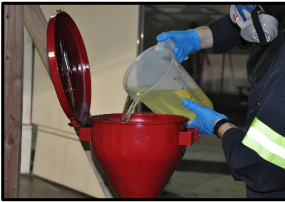
Figure 11. Gasoline being poured into barrel funnel of fuel delivery system (326975_1121770.jpg).
