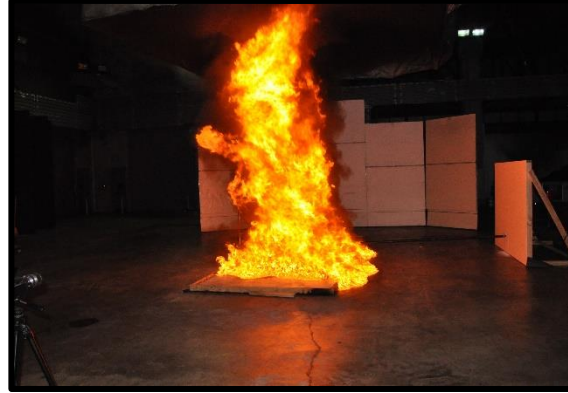
Figure 14. Resulting fire from application of torch to gasoline spill (326975_1121790. Jpg).
