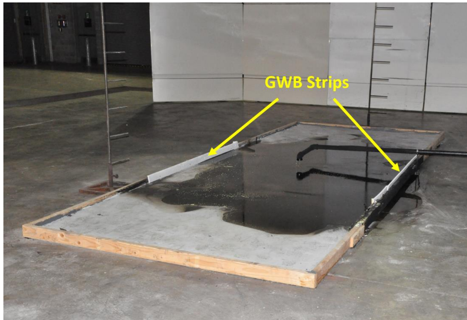
Figure 18. Strips of GWB placed at edge of pad (cropped and annotated from 326961_1121405. jpg).
