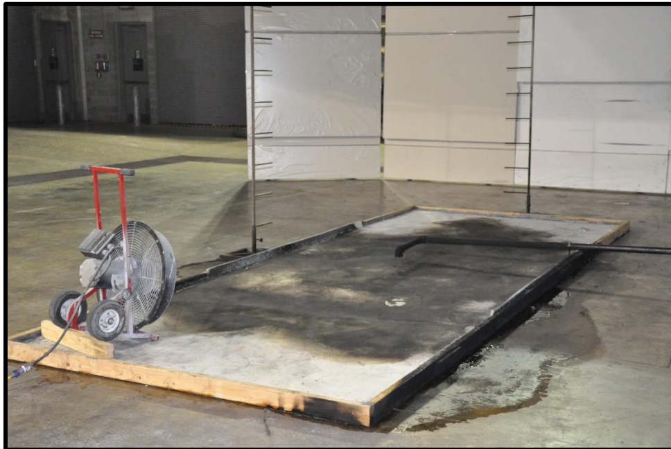
Figure 15. Fan being used to cool surface of the pad post-test (326975_1121815
