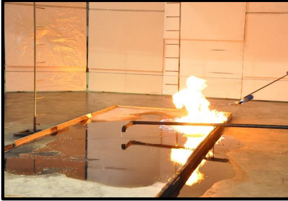
Figure 13. Application of torch to gasoline spill (326975_1121789.jpg).
