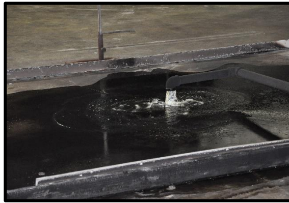
Figure 12. Fuel being discharged from delivery system onto pad (326975_1121775.jpg).
