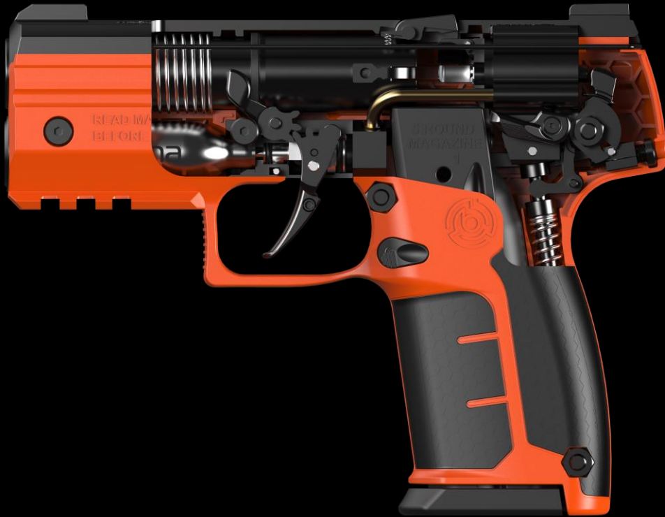
Byrna SD – Internals Cutaway
