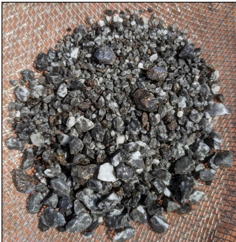
Figure 3: IQRC001 (137 to 138 metres). Sphalerite (red-brown-yellow) and galena (light grey) with associated carbonate veining within the Iroquois dolomite unit (dark grey). 12.7% Pb and 8.9% Zn.
