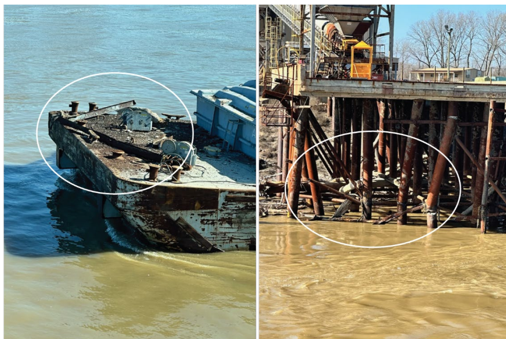
Figure 4. Left to right: The damage to barge ACBL2549 after the contact (circled), and the damage to the Port of West Memphis dock (circled). (Source: US Coast Guard)
