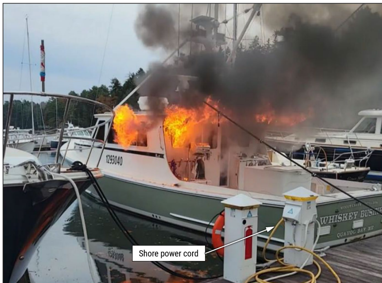
Figure 3. Fire aboard the Whiskey Business , about 0918 on November 5, 2024. Shore power cord had been connected from shore power pedestal to boat. (Background source: Mark Lenzi)
