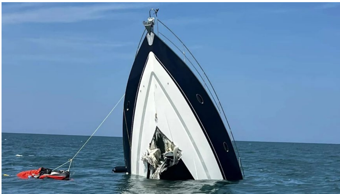
Figure 4. Hull damage to the Atlantis . (Source: St. Johns County Fire Rescue)
