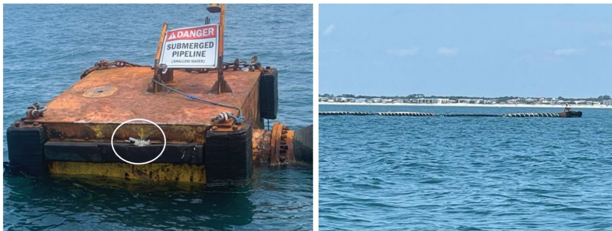
Figure 6. Left to right: The pump-out cube with damaged sign and the area where the Atlantis made contact circled; the dredge pipeline pump-out cube and floating hose from a distance, after the casualty. (Source: Florida Fish and Wildlife Conservation Commission)
