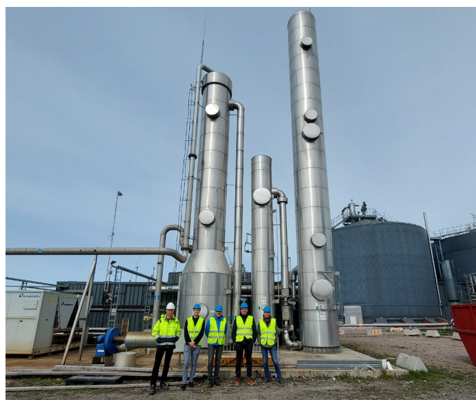
Members of the Swiss-Swedish project team in front of the Uppsala Vatten biogas plant in Uppsala (Sweden). The biogas plant separates the \text{CO}_2 from the raw biogas to produce high-quality biogas with a methane content of almost 100 per cent. Photo: OST
