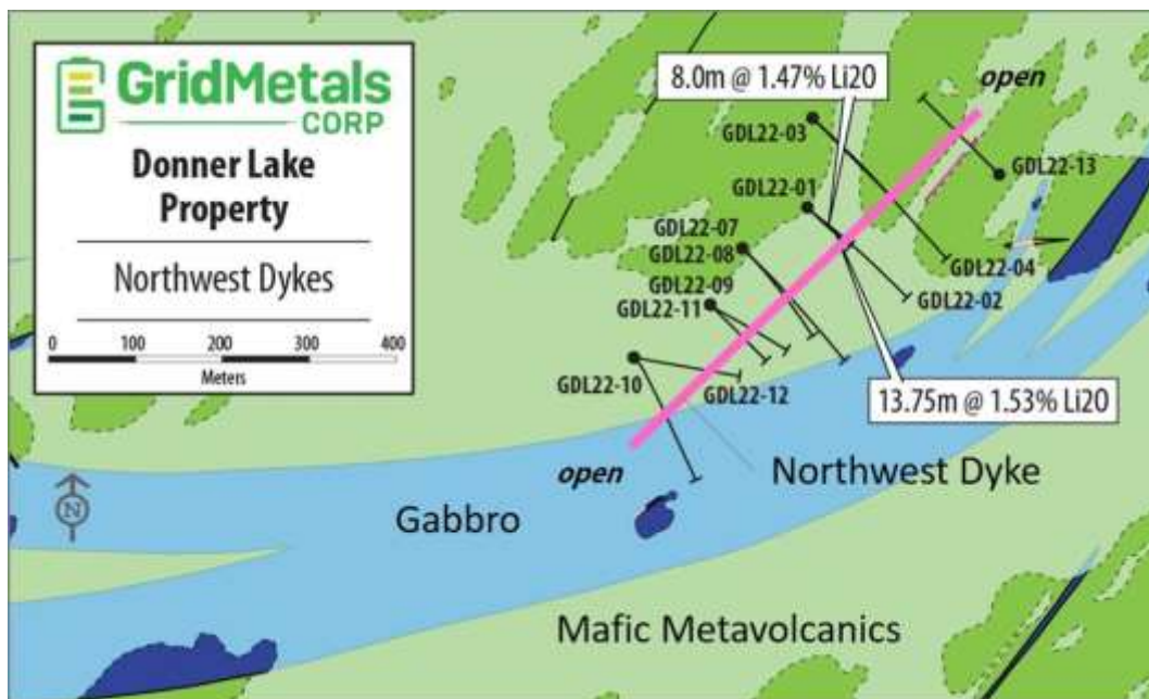
Above: location of 2022 drill holes targeting the Northwest Dyke at the Donner Lake Lithium Property
