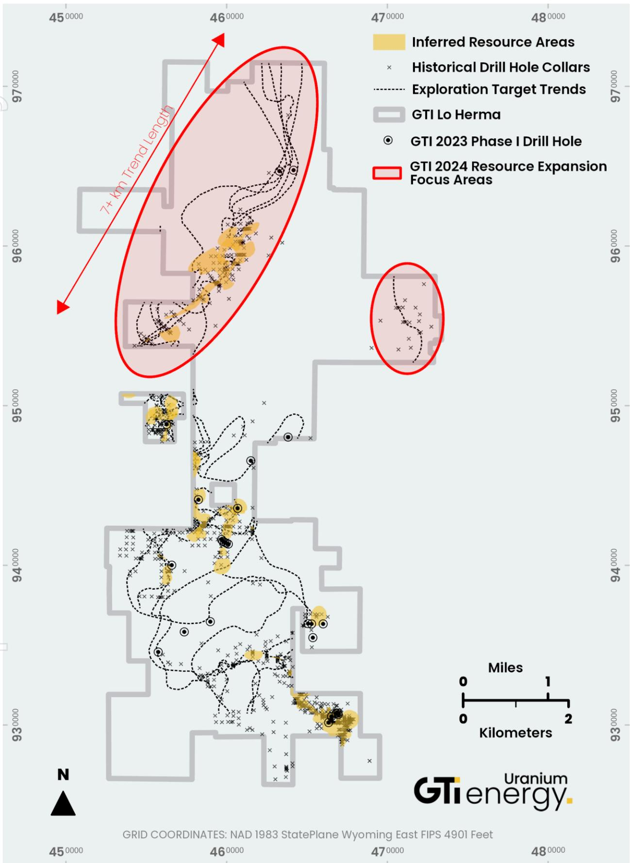
Drilling will also follow-up on drill results that have identified uranium mineralisation in the deeper sandstones of the Fort Union in the east-central portion of the project area (Figure 3).
