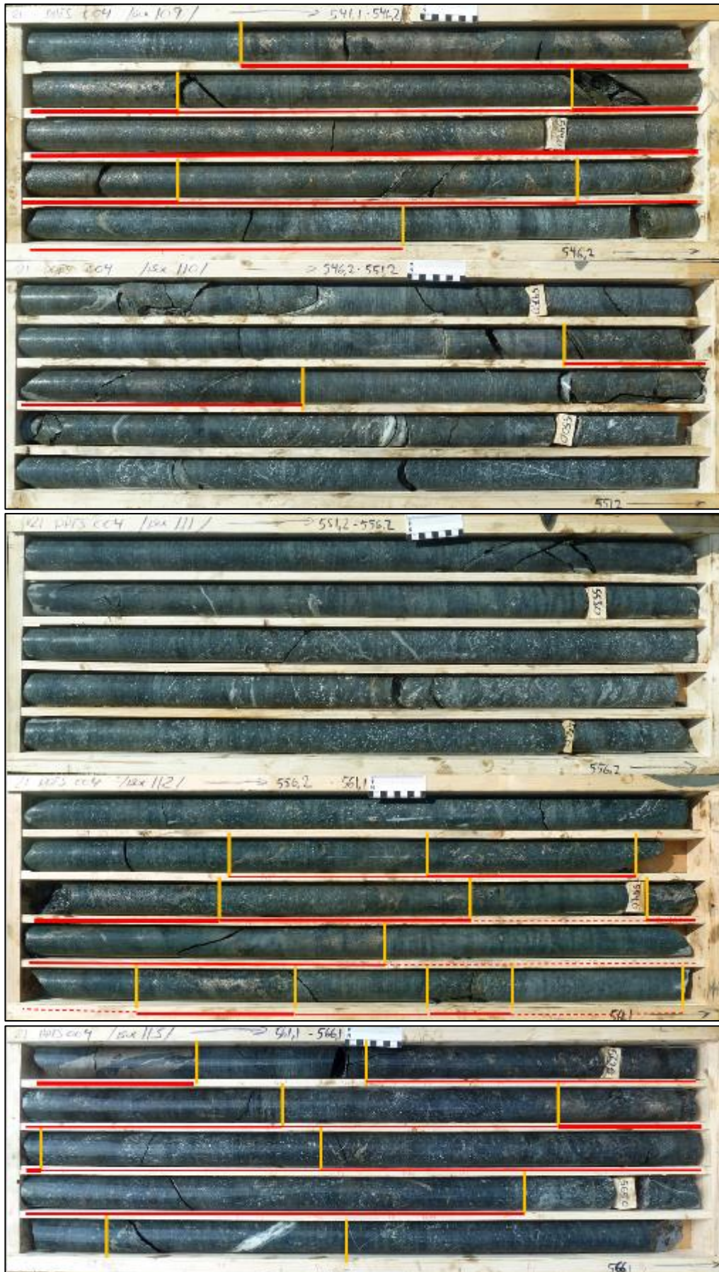
Figure 12: 21DDTS004 Central & Lower Mineralised Sulphide Zone (Trays from 541.1m-566.1m)
