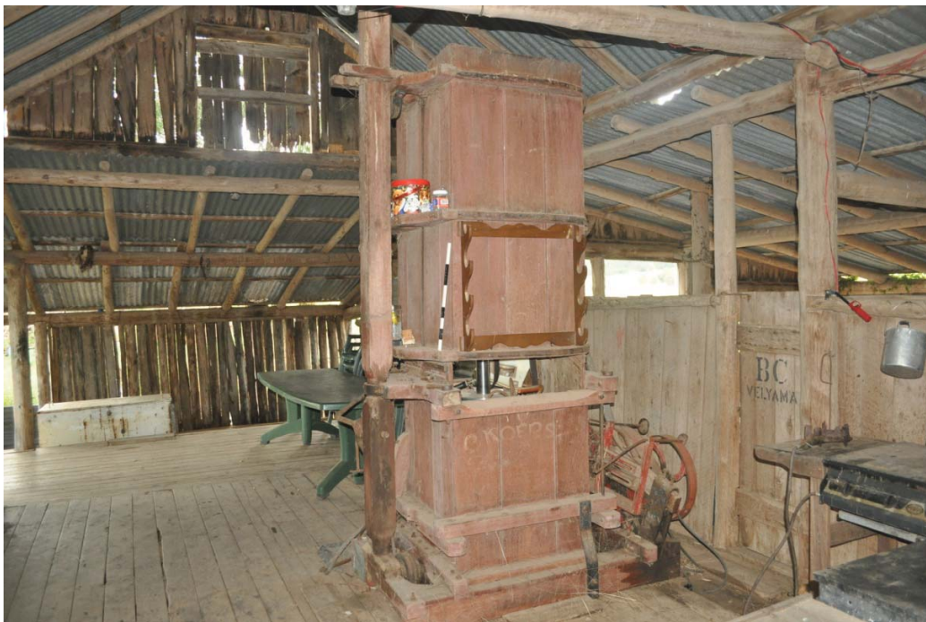
Figure 29: Wool bale press, manufactured by Christian Koeretz, Waterloo, Sydney c.1900 in the Velyama woolshed. Note the wool bale mark on the pen gate.
