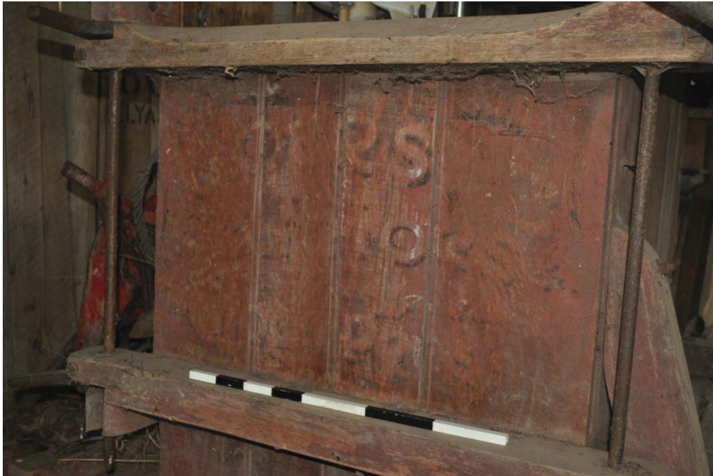
Figure 30: The middle section of the C. Koerstz wool press bearing the manufacturer's mark.
