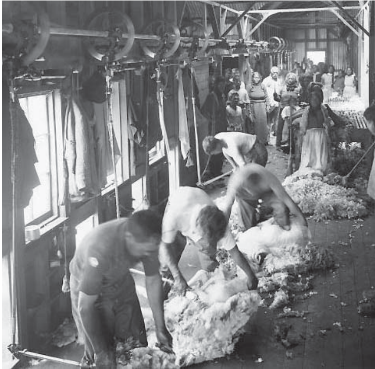
Figure 25: An example of a Lister shearing plant in operation c.1910.
