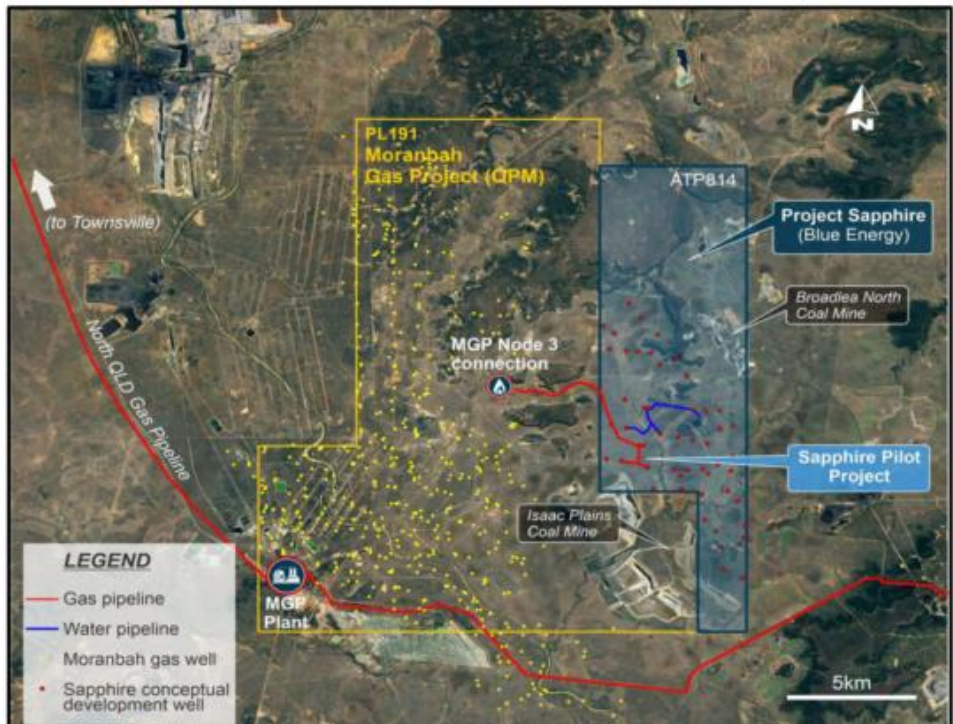
Figure 1 : Sapphire block of ATP 814 in relation to the Moranbah Gas Project and the related gas producing wells. Also shown is the proposed pipeline connection from Sapphire to the MGP Node 3 connection and initial proposed Sapphire development. Source : Blue Energy.
