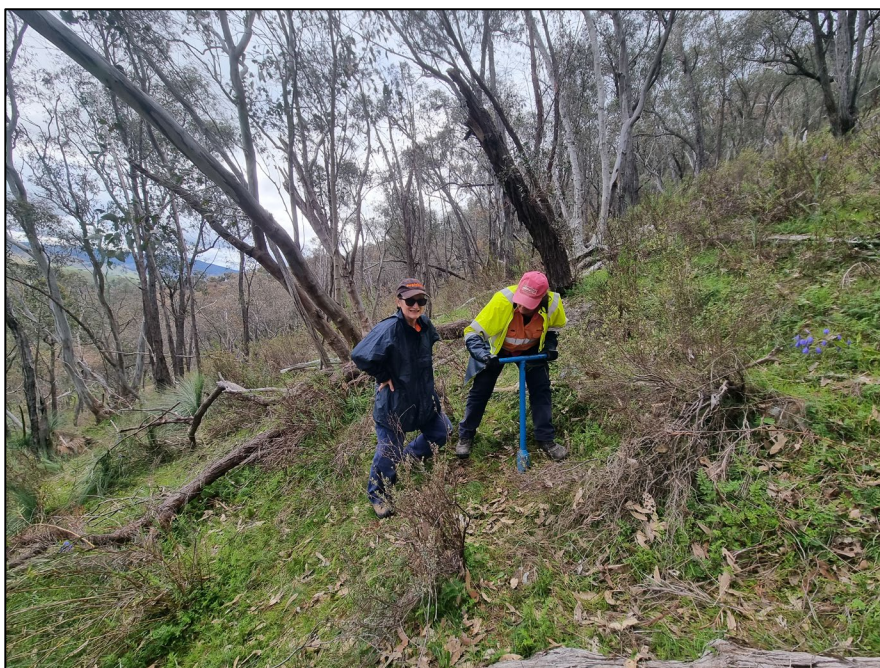
Figure 3 – Augering sample CM24-13 which contained 3.03 g/t gold. The soil sample was collected at 0.15cm depth.
