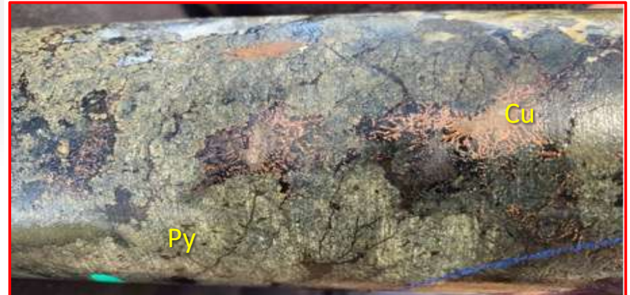
BOTTOM - TRDD001: Semi-massive pyrite (Py), disseminations of chalcopyrite and native copper (Cu) in a skarn zone from TRDD001 with 1m @ 4.24 g/t Au and 1.6 % Cu from 60.6m.
