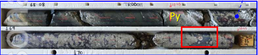
ABOVE - TRDD011: Skarn zone massive sulphide with bornite (Bn) and pyrite replacing garnet within 14m @ 1.39 g/t Au, 1.69% Cu from 58m, including 4m @ 3.36 g/t Au, 4.98 % Cu from 68m (right).
