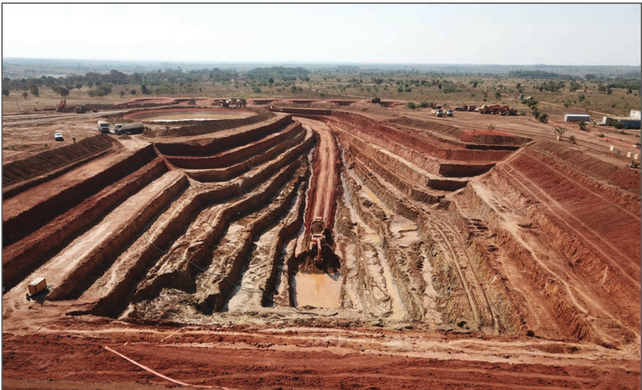
Figure 2: Kasiya Pilot Phase Test Pit mined to 20 metres depth
