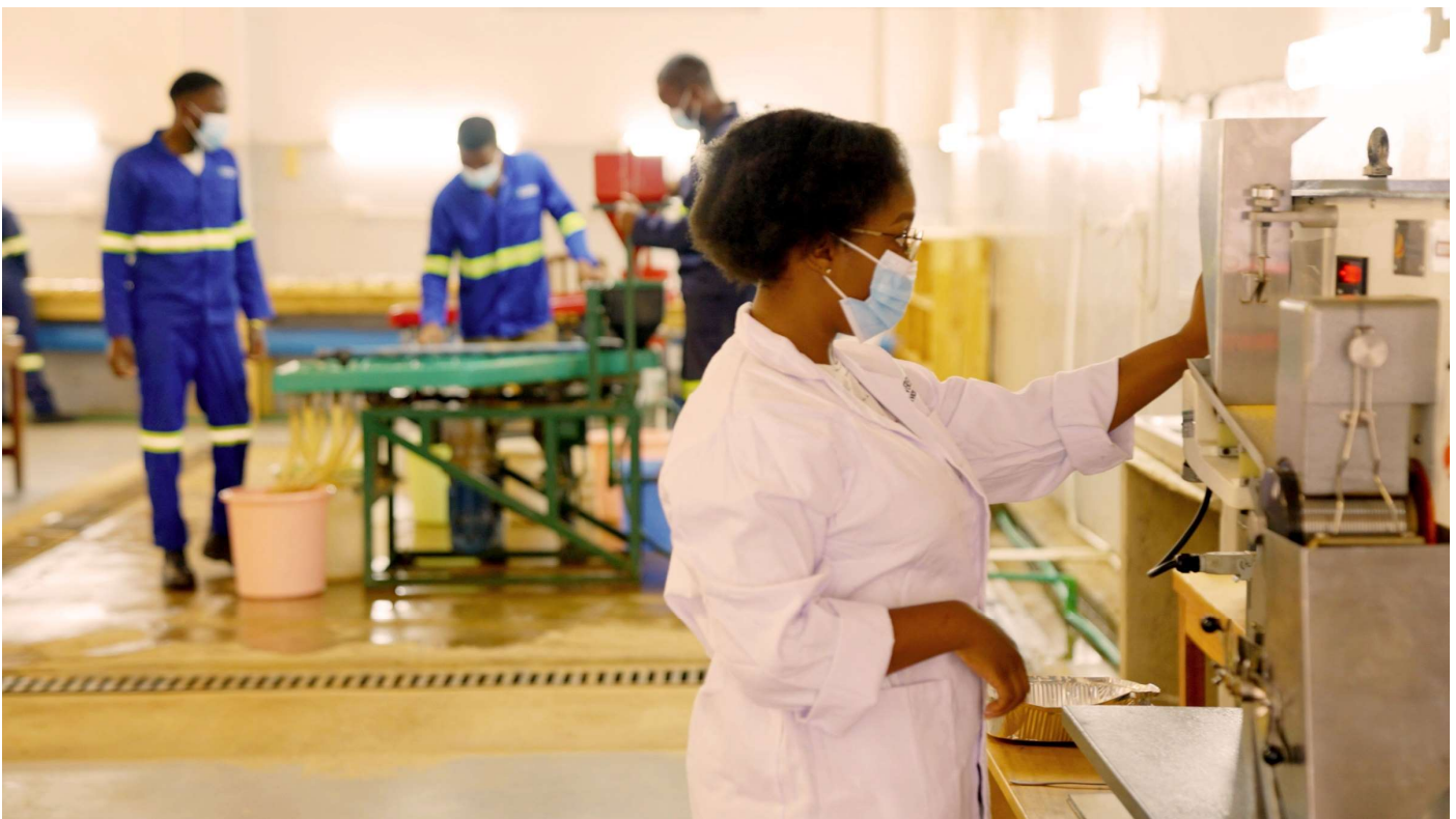
Figure 2: Wet-tabling (background) and magnetic separation (foreground) at the Company's established laboratory in Malawi
