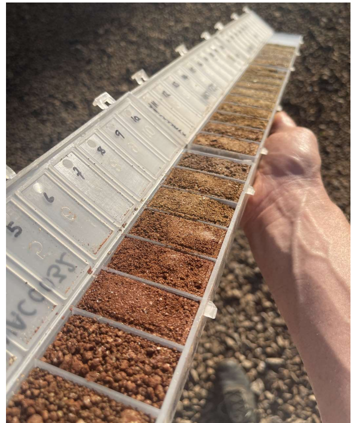
Figure 9 & 10: Kasiya drilling sample collection under the cyclone and mineralised weathering profile displayed in a chip tray
