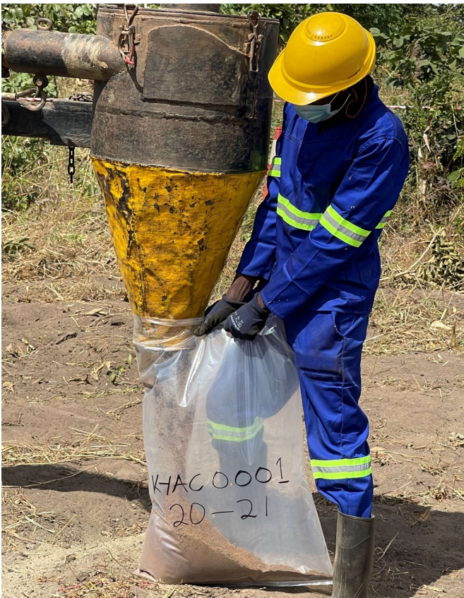
Figure 9 & 10: Kasiya drilling sample collection under the cyclone and mineralised weathering profile displayed in a chip tray
