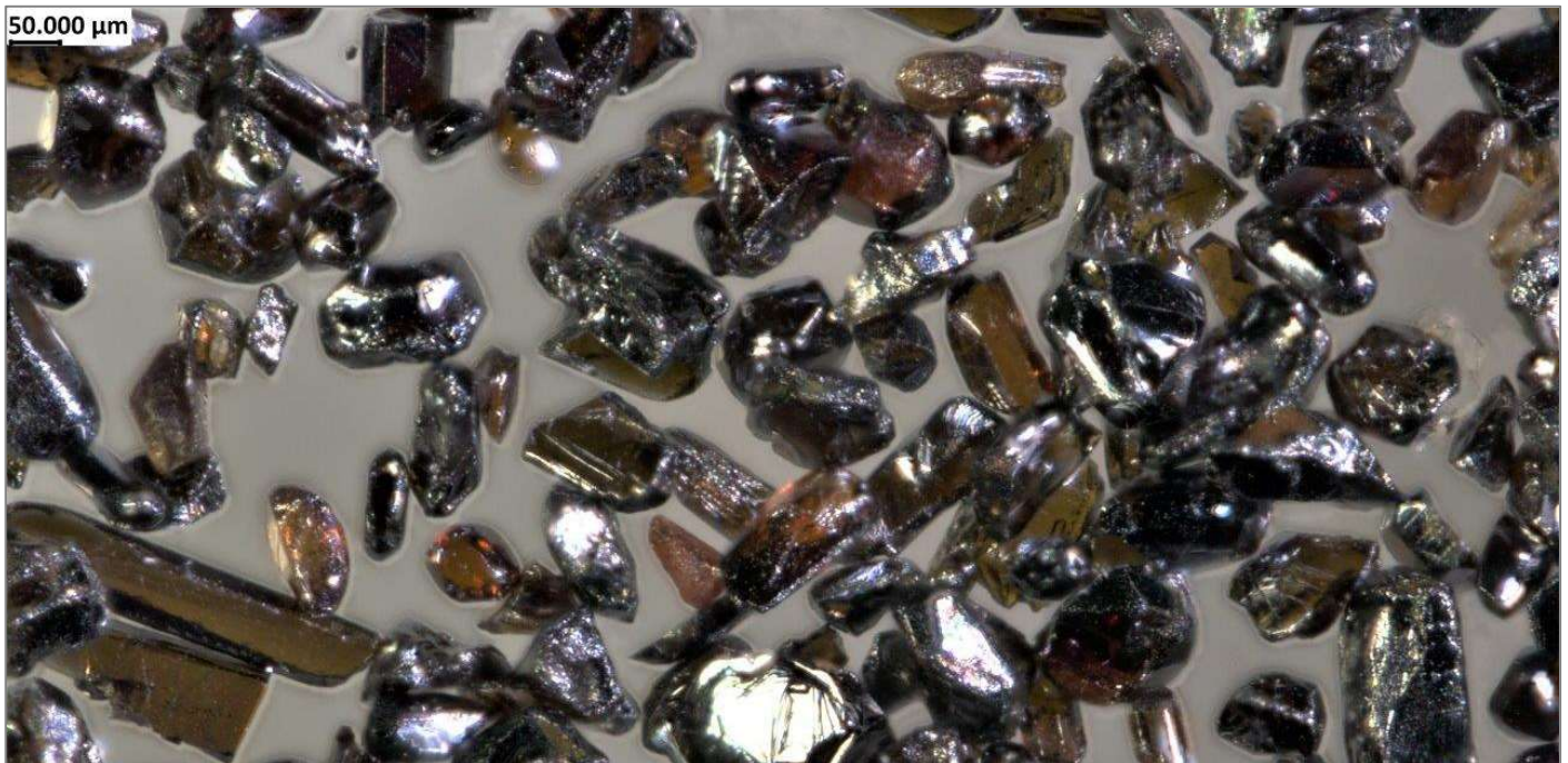
Figure 7: Photomicrograph of high purity rutile product 97.2% TiO 2
