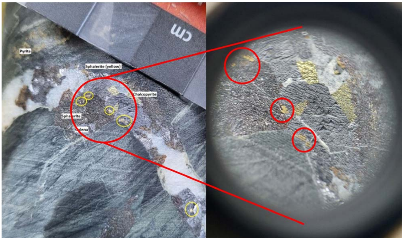
Figure 7. Visible gold. Sheeted calcite-sulphide-gold vein in HQ3 core (left) with a 20x magnification hand lens view (right), 405m in BD22004.
