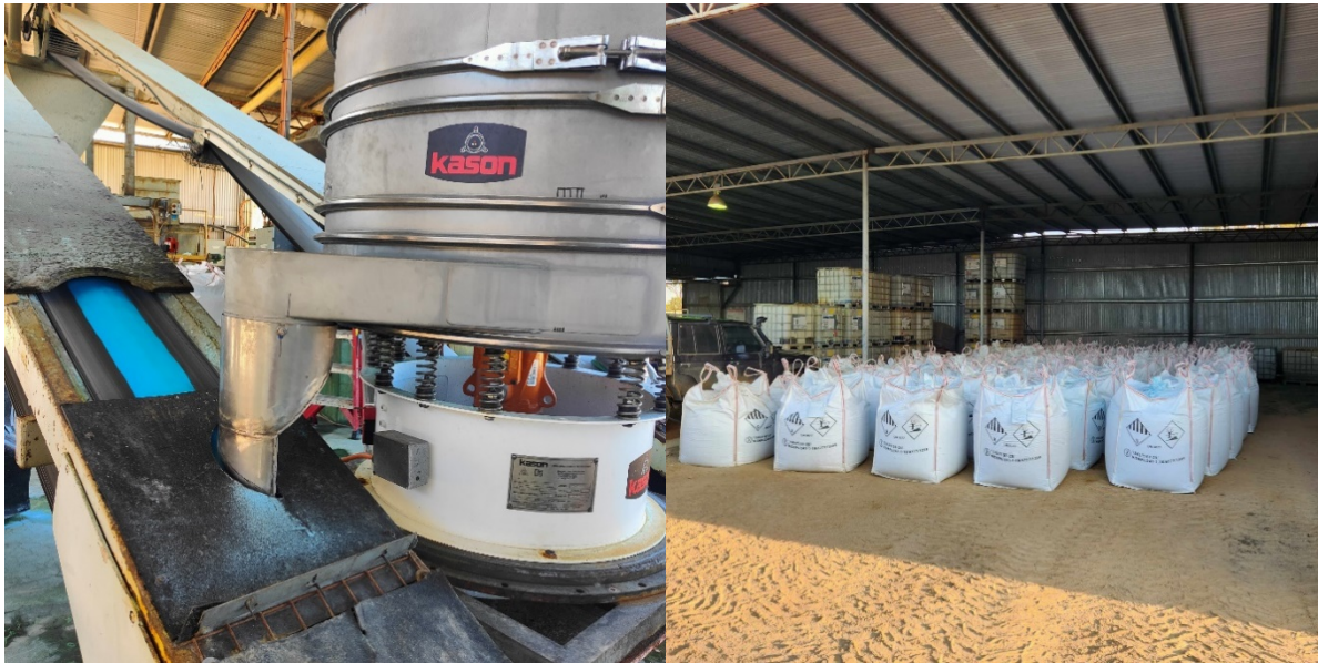
Figure 3. (a) Screening of copper sulphate pentahydrate prior to bagging. (b) Copper sulphate pentahydrate bags ready for collection.
