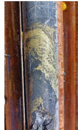
Figure 5. (a) Oxide, transitional and primary (fresh) resource estimation for the Tartana open pit using inverse distance estimation and a 0.2% Cu cutoff grade. (b) Primary copper mineralisation from drillhole D15.
