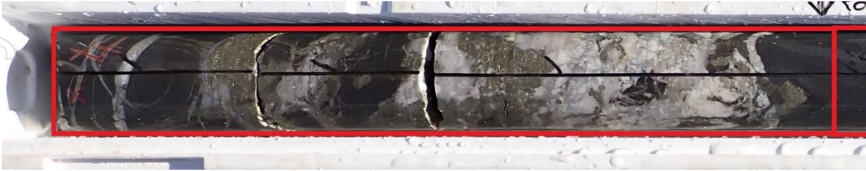
Figure 2: Example of sulphide mineralization in brecciated rock yielding 1.62g/t gold in drill hole PDD0001.
