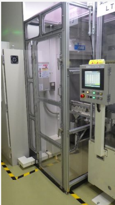
Production equipment placed in airtight booths
