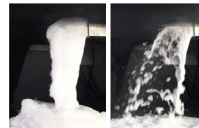
Foam fire extinguishing agent developed by Nohmi Bosai (left) and conventional commercial product (right)
