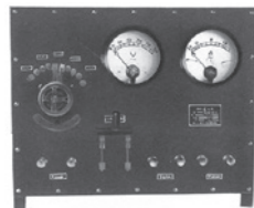
Choke coil auto transformer
