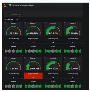
EoM management console, in which the user is able to check the amount and type of data, and to identify the ports where problems such as packet drops are occurring.
