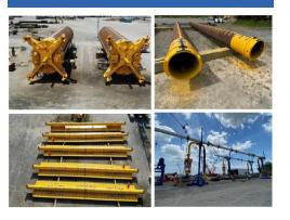
Structures associated with a Gulf of Mexico subsea development consisting of Suction Piles, Sleepers, Mudmats, Jumpers and PLET pin piles.
