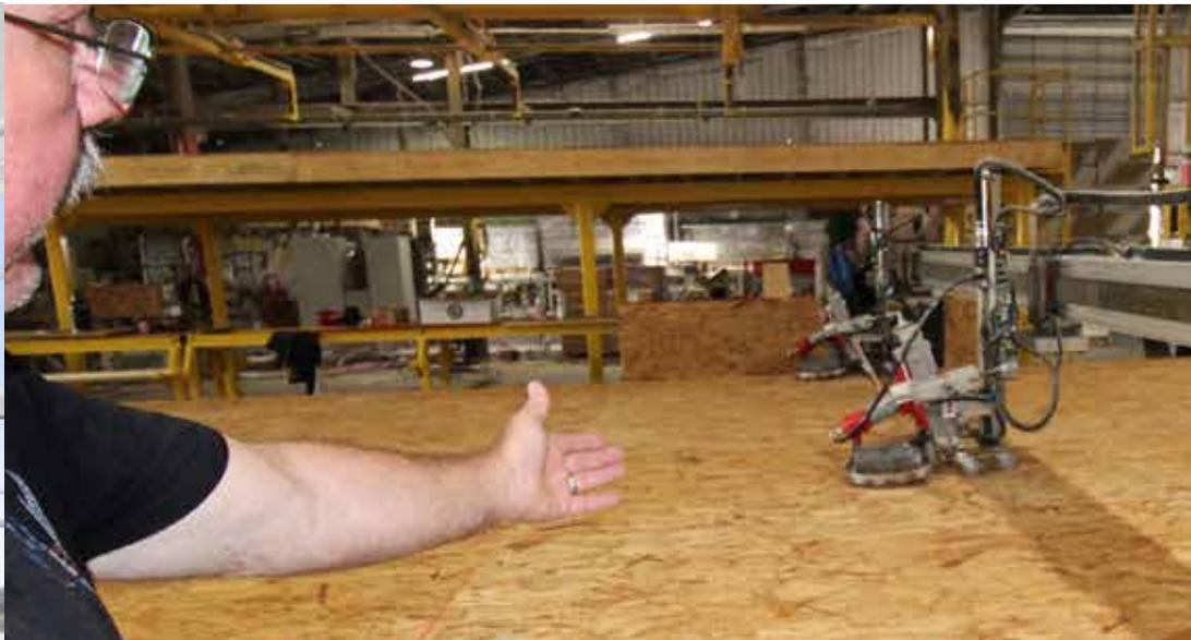
The gantry gun is an automatic dual nail gun system that provides speed and guided precision to nailing sub-flooring panels to floor joists.
