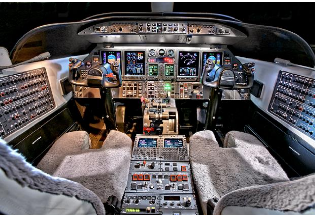
Traditional Cockpit with Mechanical Circuit Breakers Learjet 45
