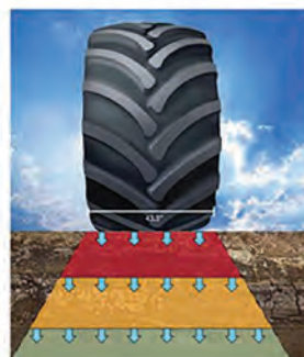
▲ SUPER SINGLE SETUP COMPACTION
