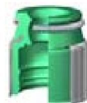
Under pressure, the lip of a conventional valve stem seal opens, which means that lubricating oil escapes and the valve guide shows excessive wear as a result. The high-pressure valve stem seal does not open and so wear is kept to a minimum.
