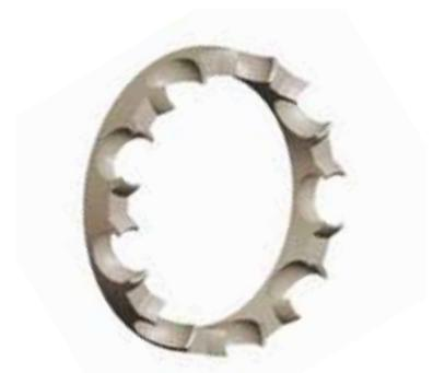
**NUBS (non uniform ball spacing) cage** for deep groove ball bearings prevents the hooting noise during cold starts. The cage is designed especially for use in bearings for alternators, starter-alternators and electric traction motor bearings for hybrid and electric vehicles.
