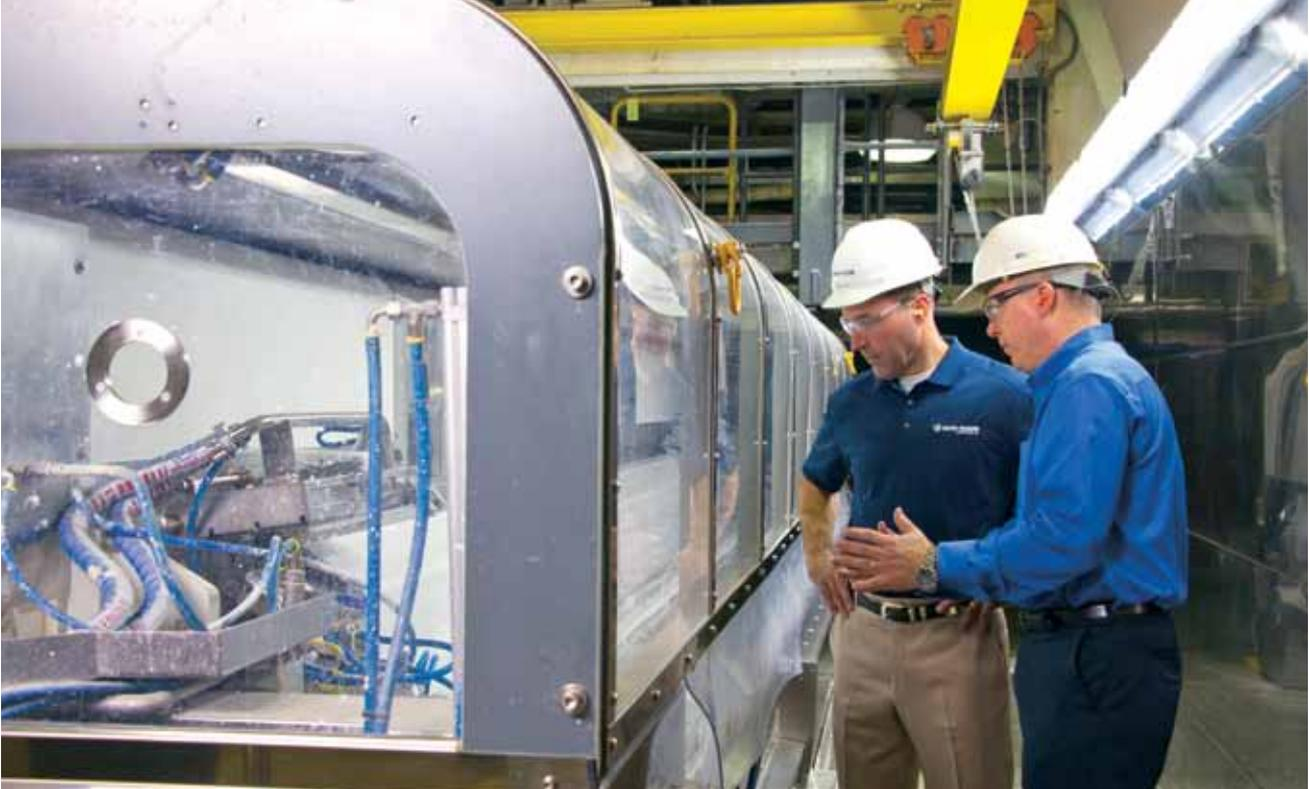
**Curtain Coater:** We invested \$30 million to add a curtain coater to our number one paper machine in Macon, Georgia. As a result, we materially reduced our usage of  $TiO_2$ , which significantly increased in price during 2016.
