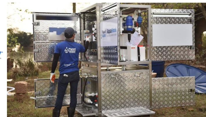
AquaBlock with Dosatron D14MZ1000 pumps
