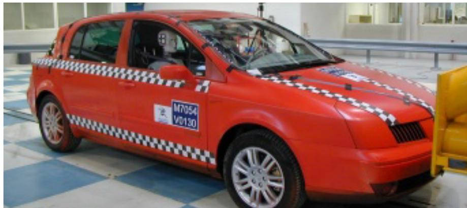
Autoliv France has expanded its technical center by adding a new track for full-scale test where complete vehicles, weighing up to four tons, can be crash tested at speeds up to 80 km/h or vehicles weighing two tons can be tested at 120 km/h. The tests are not only frontal, but also rear, side and car-to-car. Since the opening in May 2000, more than 150 full-scale tests have been performed in the new crash lab.
