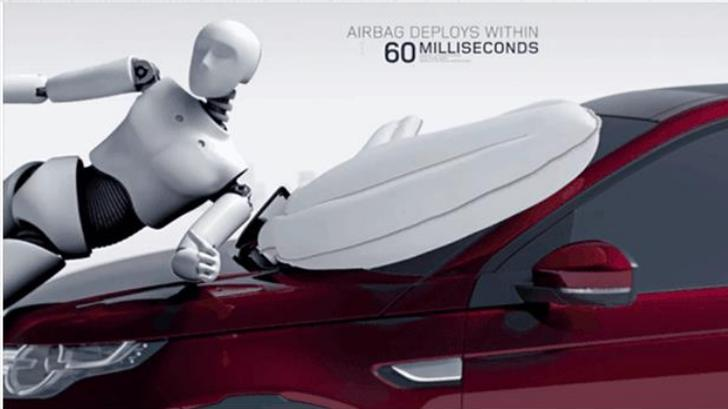
🚗 Pedestrian airbag improves head protection for vulnerable road users around the windshield
