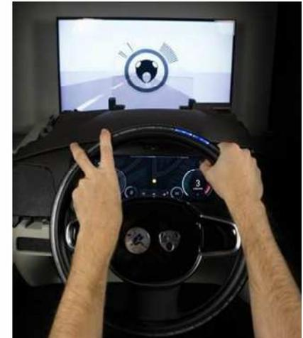
High resolution sensor with the option to create virtual buttons using the sensor RGB LED's
