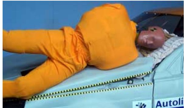
*Autoliv's Active Hood (left) and Pedestrian Protection Airbag (right) improve the safety for pedestrians by reducing the risk of a person hitting the hard car structure, the base of the windshield or the windshield pillars.*
